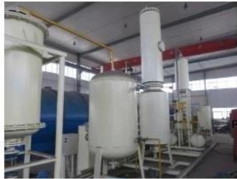
Pyrolysis oil distillation plant
