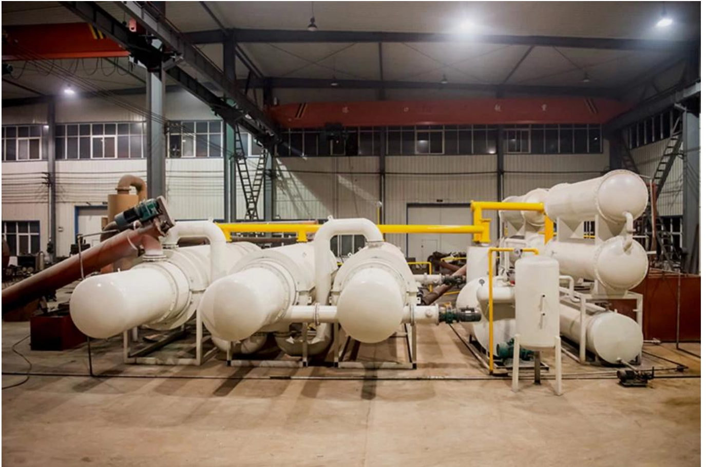
2018 fully continuous plastic pyrolysis plant recycling to fuel oil
