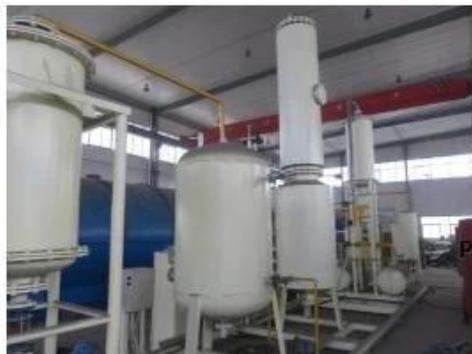
Pyrolysis oil distillation plant
