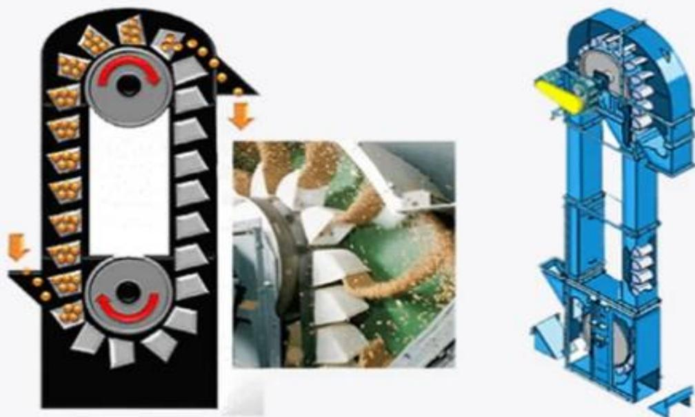
Work in a fully enclosed enclosure to ensure that the process of lifting and conveying is unobtrusive, and the environment of the entire lifting and conveying process is guaranteed to be hygienic and pollution-free
